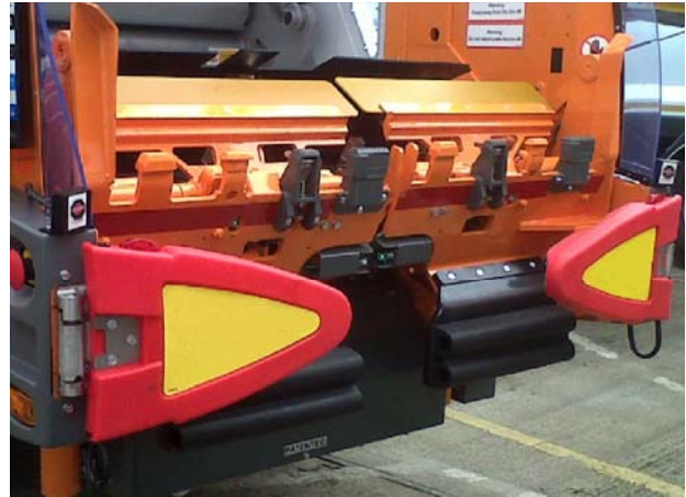
Sentinel Systems has developed a new and advanced radar system designed to detect pedestrians, cyclists or buildings by causing the vehicle to automatically brake if an obstruction is detected within a predetermined range.
