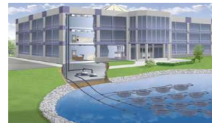
Surface water (closed loop)
