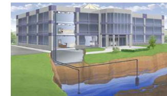
Aquifer or mine water (open loop)
