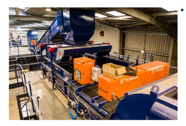
This TOMRA allowed a further split of the mixed plastic fraction to drive out flexible plastics and Polypropylene (as well as the existing PET & HDPE).
