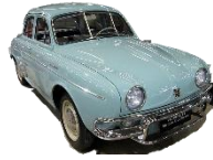
HENNEY KILOWATT DAUPHINE WITH 60 MILES AUTONOMY
