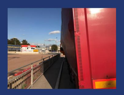
This is a vehicle encountered at the Dartford Crossing Check Site in Kent. As you can see from the photos, the whole vehicle is leaning to one side. When this was inspected, the cause was found to be a suspension airbag which had blown mid-journey. Due to the load being insecure, once the airbag blew it shifted the whole load.
