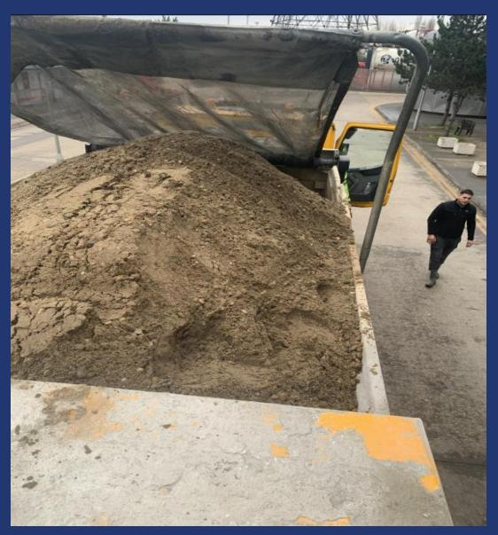
Volumetric mixer overloaded and insecure load.
