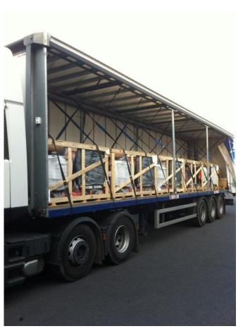
Loads carried in <u>standard</u> curtain-sided vehicles should be secured appropriately, without using the curtains as part of the securing system
