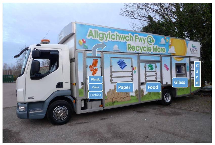
33m³ usable body volume on DAF LF45 5000mm wheelbase, 12 tonne GVW, 3.7 tonnes payload
