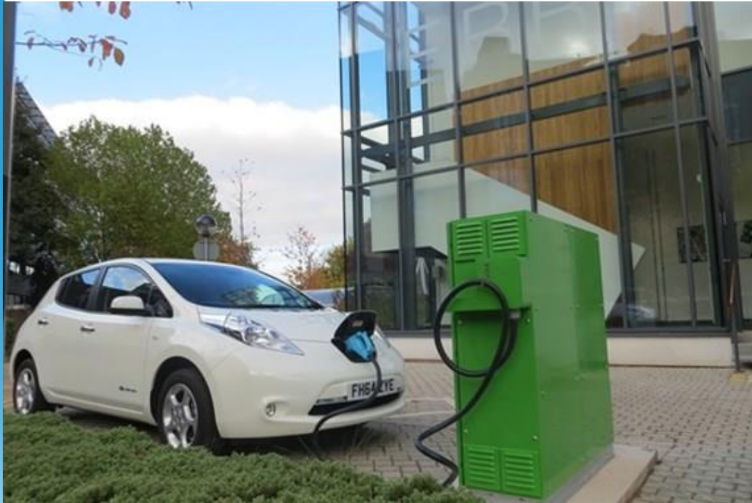
Cenex installed the UK's first installed V2G unit at Aston University. Storing cheap night time electricity from on site CHP scheme run by Engie.
