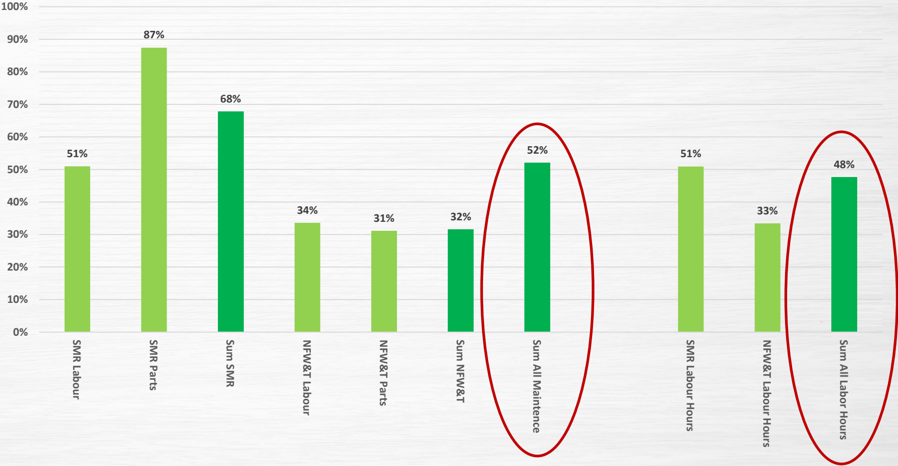
BEV Maintenance Costs & Labour Hours % Reductions Combined Years 1&2
