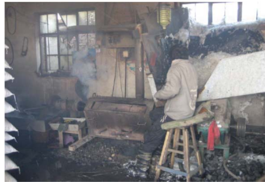
“Coal fired extruder in a small recycling plant in China.” After (Jefferson 2010)
