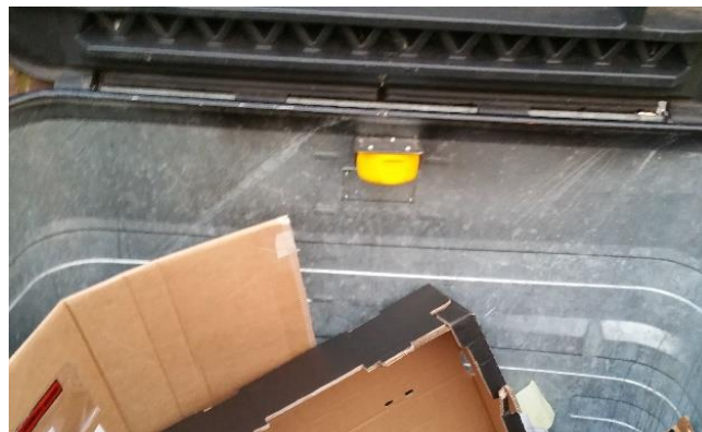
(Fig 5) Possible cause of false sensor reading
