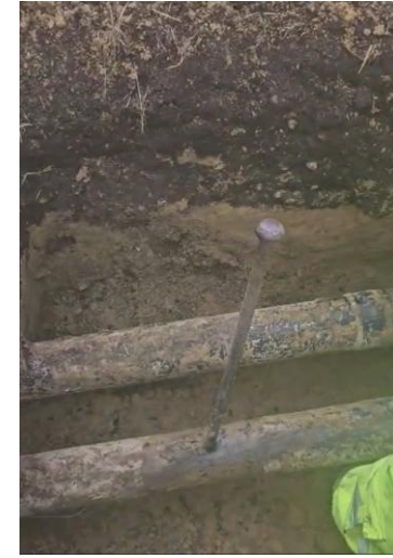
Left: heat network pierced by marquee, right: Power cable failure
