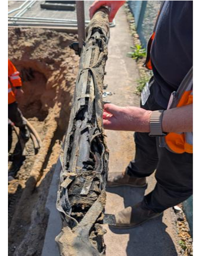
Left: heat network pierced by marquee, right: Power cable failure
