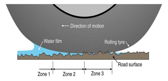
Zone 1: Continuous water film Zone 2: Interrupted water film Zone 3: Dry contact
