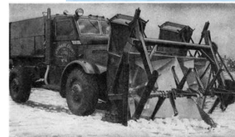
The rotating larks at the front end of this machine break down any kind of snow bank and feed it to blowers which throw it well off to one side
