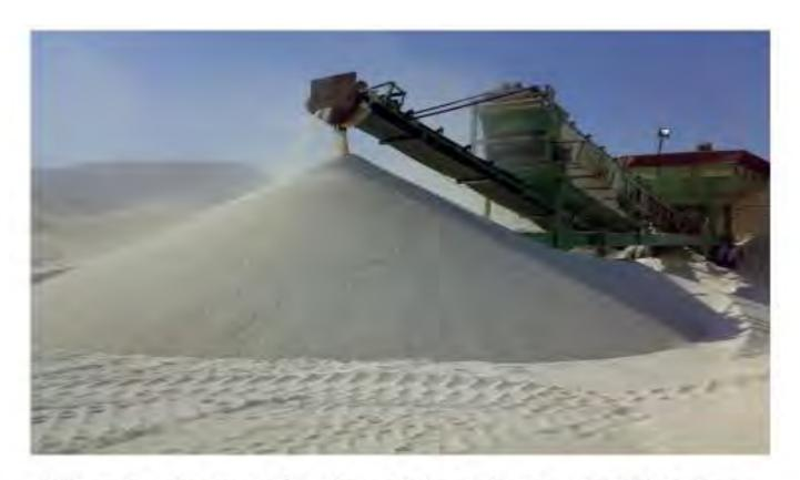
Silica sand, soda ash and limestone are the main raw materials for glass. The acquisition causes environmental damage and melting them together uses a lot energy resulting in high levels of carbon emmissions.
