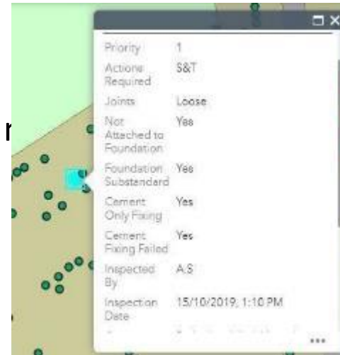
Internal Collector View of Inspection result
