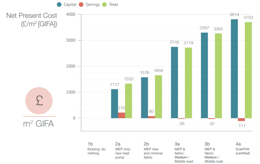
Graph 20 / Net Present Cost of retrofit showing offset of capital investment over the next 30 years (£/ year).
