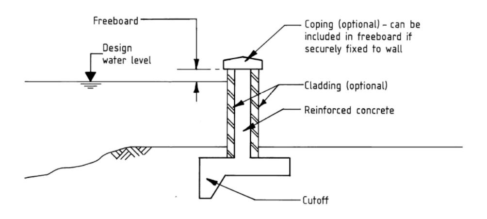
Figure 9.3 Typical floodwall
