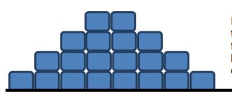
Pyramid/terraced storage of bales may lessen the risk of a bale falling during a fire resulting in fire spread. However, this method may increase bale footprint relative to volume and may cause operational handling issues
