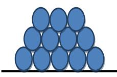
Round/tubular bales and loose materials which may roll should a stack collapse during a fire may result in fire spread – such factors need to be taken into account in your calculations to arrive at separation distances
