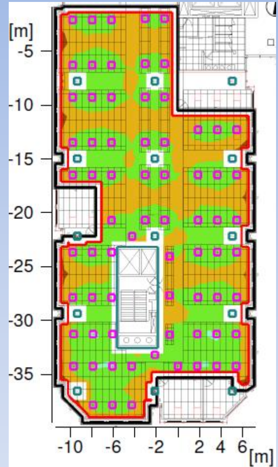
Lighting design by Council engineers for Civic Offices showing proposed lux levels from LED lighting
