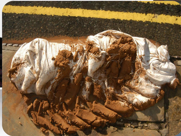
Sandbags – largely ineffective
