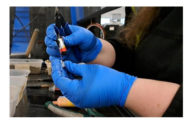
Batteries can be safely removed by hand.
